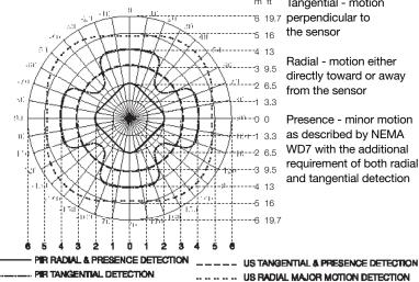
m ft Tangential - motion 19.7 perpendicular to the sensor
